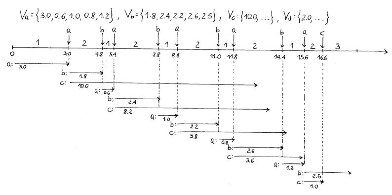
Four jobs are completed (events b') before the machine breaks down for the first time (event c'),
