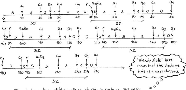
1. The discharge time of the battery at steady state is 32 min.
