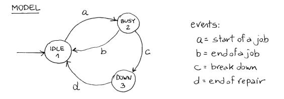
WARNING: the clock of event 'c' is restarted in state Busy and stopped instate IDLE; moreover, the clock of event 'c' is reset to zero in state DOWN.
