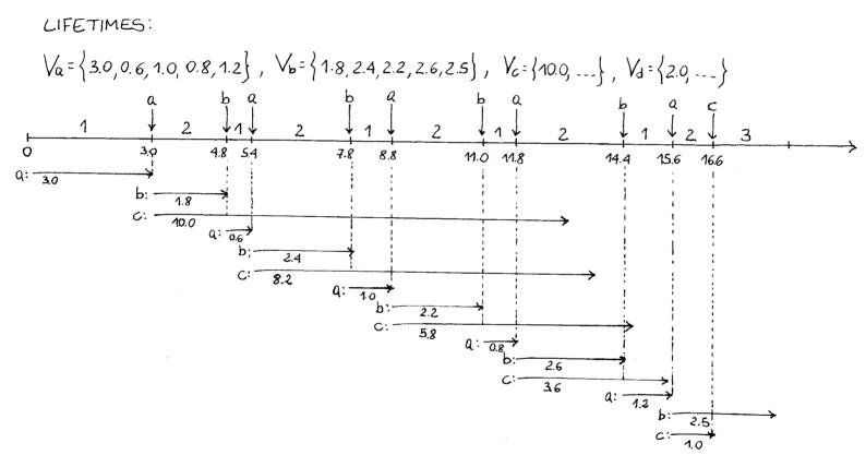
Four jobs are completed (events 'b') before the machine breaks down for the first time (event 'c').
