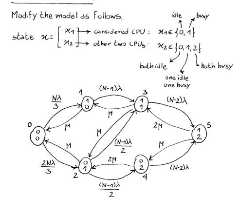
Using this model, the utilization of the considered CPU is:  $U = TI_1 + TI_3 + TI_5 \simeq 0.3049$
