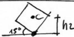
$$\Delta U = Mg(h_2 - h_1) = Mg\left(\frac{\sqrt{2}}{4}L - \frac{L}{2}\right) = \dots$$
