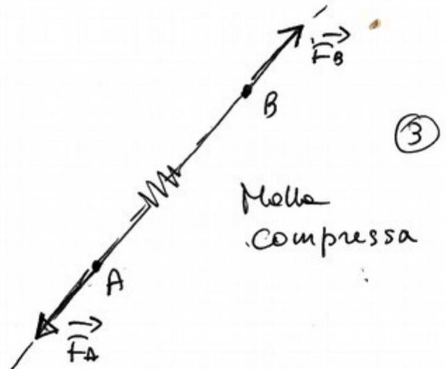
$$\left. \begin{aligned} \vec{F}_A &= |\vec{F}_A| \cdot \vec{e}_{AB} \\ \vec{F}_B &= |\vec{F}_B| \cdot \vec{e}_{BA} \end{aligned} \right\} \textcircled{1}, \textcircled{2}$$
