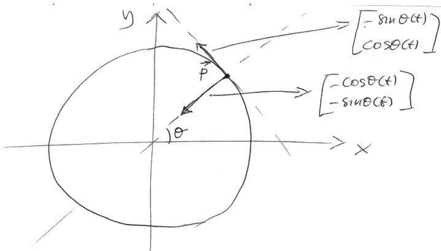
$$\vec{a}(t) = R\omega^2(t) \begin{bmatrix} -\cos\theta(t) \\ -\sin\theta(t) \end{bmatrix} + R\alpha(t) \begin{bmatrix} -\sin\theta(t) \\ \cos\theta(t) \end{bmatrix}$$
