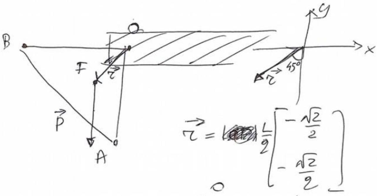
$$\begin{aligned}\tau_z &= r_x P_y - r_y P_x \\ &= -\frac{L}{2} \frac{\sqrt{2}}{2} (-Mg) = \frac{L \sqrt{2} Mg}{4}.\end{aligned}$$
