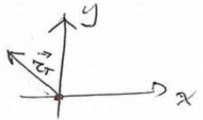
$$\vec{r}_T = L \begin{bmatrix} -\cos 45^\circ \\ +\sin 45^\circ \end{bmatrix} = L \begin{bmatrix} -\frac{\sqrt{2}}{2} \\ \frac{\sqrt{2}}{2} \end{bmatrix}$$
