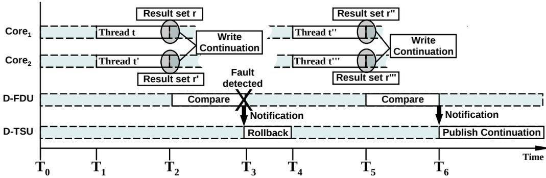
**Figure 3: Example for a recovery scenario.** Thread  $t$  is duplicated as  $t$  and  $t'$ . After the execution both thread instances write back their result set, which are compared by the D-FDU (at  $T_2$ ). In the case of a transient fault, the D-TSU re-executes Thread  $t$  as  $t''$  and  $t'''$  again on the same cores ( $T_4$ ).
