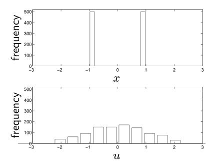
unequalized estimator  $\hat{x}(t) = \mathrm{sgn} u(t+D)$  has 19% error rate (using D=5)
