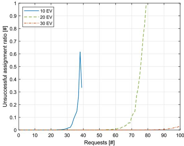
**Fig. 5.** Fraction of infeasible assignments to the total number of filtered scenarios versus the number of requests for 10, 20, 30 vehicles.
