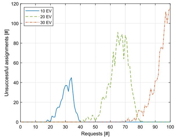
Fig. 4. Number of infeasible assignments out of the filtered scenarios versus the number of requests for 10, 20, 30 vehicles.
