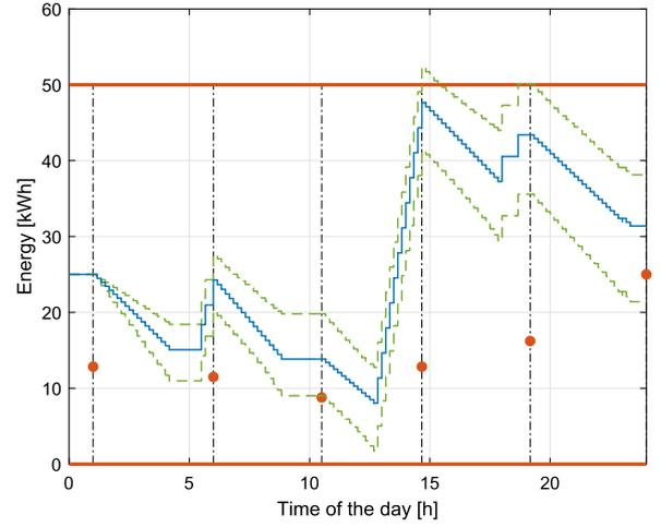
**Fig. 1.** Battery energy level profile for a simulation which satisfies all the constraints (blue solid), envelope of all the battery energy level profiles over  $N = 10^4$  simulations (green dashed), capacity constraints (red solid), and request constraints (red dots). (For interpretation of the references to color in this figure legend, the reader is referred to the web version of this article.)
