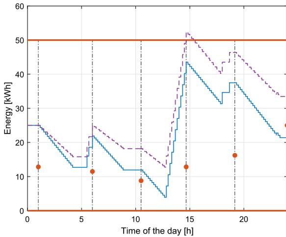
Fig. 2. Battery energy level profiles for a simulation which violates the terminal constraint (blue solid) and for another which violates the capacity constraint (magenta dashed), capacity constraints (red solid), and request constraints (red dots). (For interpretation of the references to color in this figure legend, the reader is referred to the web version of this article.)
