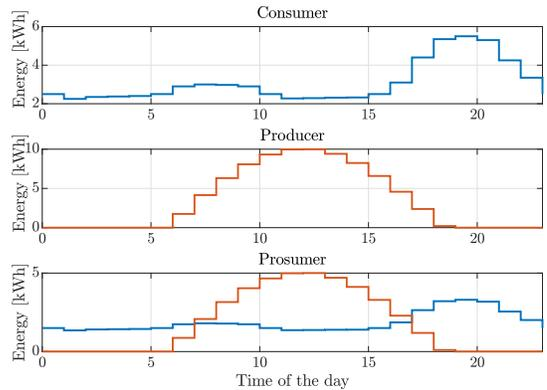
Fig. 1. Load (blue) and generation (orange) profile of the consumer, producer and prosumer of the community.
