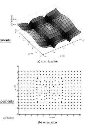
Fig. 4. The cost function (17) and the associated orientations for a four landmark scenario.
