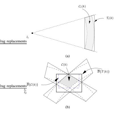
Fig. 2. (a) Trapezoidal approximation of a sector of corona. (b) Outer approximation of the exact feasible position set C(k) (dashed region) related to two landmarks.
