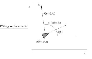
Fig. 1. Range and bearing measurement with respect to the *i*-th landmark.
